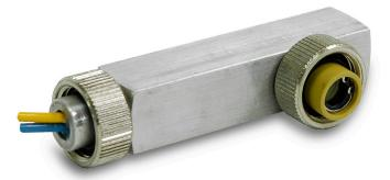
This sensor features a high sensitivity ultraviolet (U.V.) tube for monitoring gas or oil flames that cycle on and off frequently. The Eclipse flame safeguard checks for a short-circuited, or "runaway" scanner at the beginning and end of each flame cycle.
